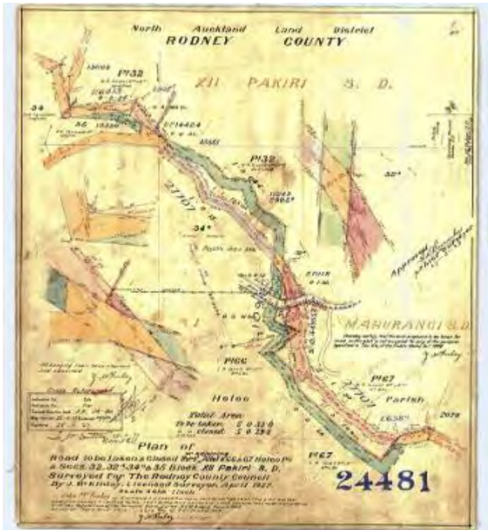
Figure 64 – Plan of SO 24481 showing the planned road deviation
