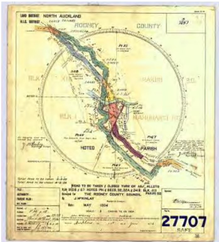
Figure 65 – Plan SO 27707 dating to 1934 with the road deviation shown
